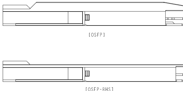
Figure 9-1: Side view of a typical OSFP (top) and a typical OSFP-RHS (bottom)
