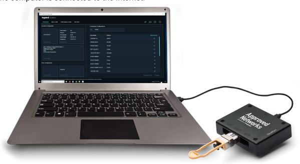
Connect the OnePort Programmer unit to the computer with the included USB cable. If the OnePort Programmer's USB port successfully establishes a connection to the computer, the USB connection icon will be green. Otherwise, the USB Connection icon will turn red, and the error message "Please Connect OnePort Programmer" will pop up. Make sure connections are secure and check the troubleshooting section of this guide if necessary.
